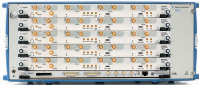
Figure 20. Five Agilent M9703A AXIe 12-bit digitizers installed in the Agilent M9505A 5-slot AXIe chassis to form a 40-channel 12-bit acquisition system.
